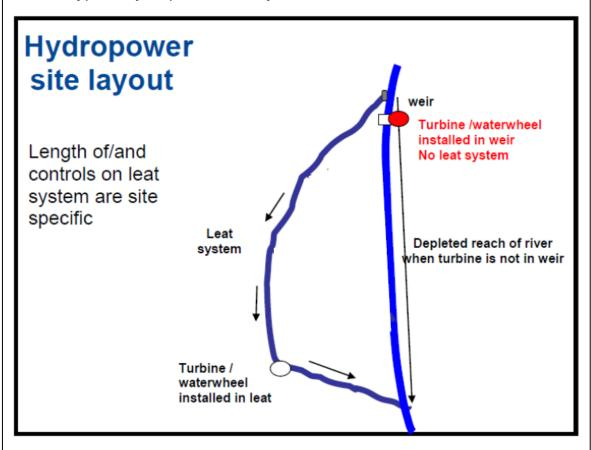
Hydropower site layouts vary, but many of the main elements are shown Figure 1. A weir (impoundment) is present in almost all hydropower sites, and may provide the head drop of water on its own, or in conjunction with a fall in the river over a greater length.
