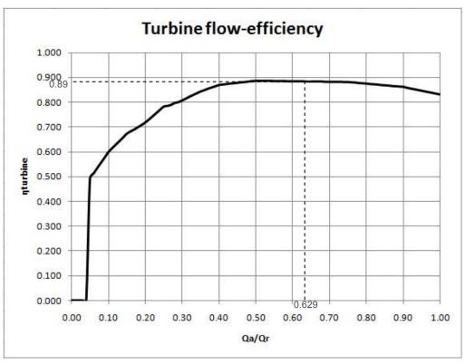
$<sup>\</sup>eta$  = efficiency of turbine, Qa = actual (measured) flow, Qr = rated flow (dashed line represents example given in 7.4.3)
